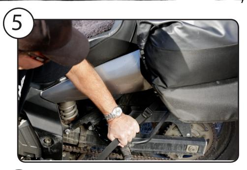
The last step for making a secure connection to the motorcycle is threading the Forward Attachment Straps to your passenger footrest bracket.
