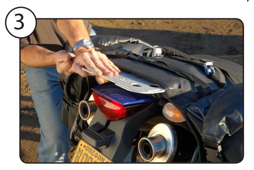
Next, thread or wrap the Rear Connection Strap around your rear luggage rack and secure that strap as tight as needed. This connection is preventing the pannier from sliding forward into the riders' area. This becomes the anchor point and the two front straps will make the system tight. Keep in mind the ideal position you wanted while tightening the straps.
