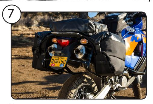
Shown on the left is the Top Case properly positioned and the Lower Side Compartments correctly secured with the ramp connected to the Upper Side Compartment roll top and the horizontal side release buckle capturing the ramp.
