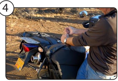
Once you have determined the correct position for the two Center Rack Attachment straps, cinch those down as tight as possible. Think about cinching a saddle on a horse - you want those very tight, they will not slip through the metal cam lock buckles. These straps create the second connection to the motorcycle and stabilize the saddlebags from lateral movement.
